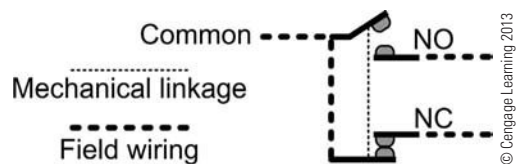
FIGURE 7-22 Class C contacts from NO and NO contacts
