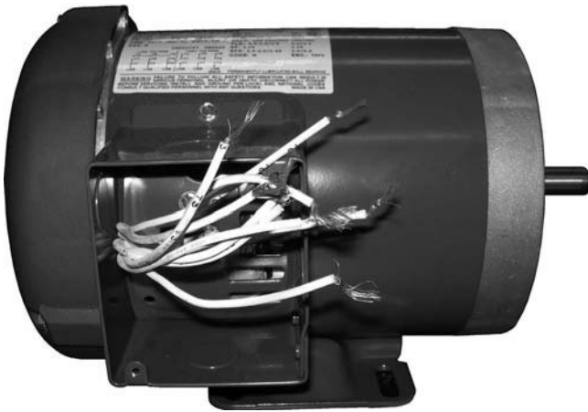
FIGURE 5-4 NEMA three-phase motor with individual connection leads
