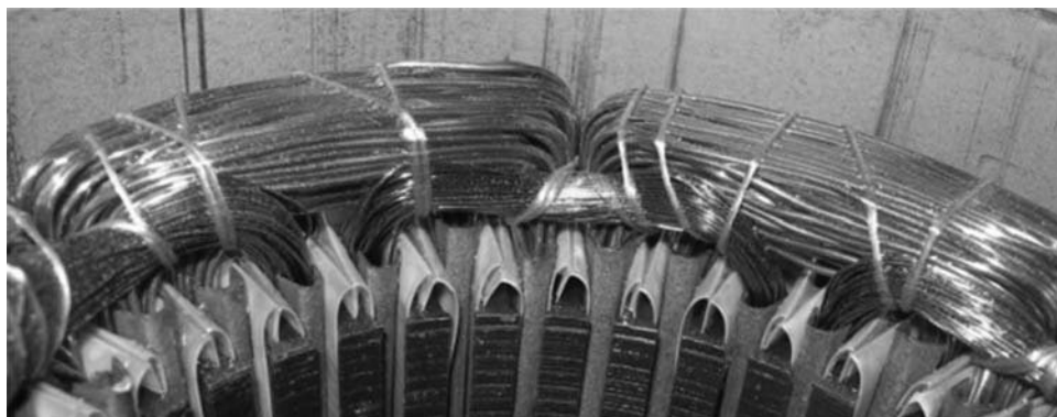
FIGURE 4-1 Main stator windings with auxiliary start windings
