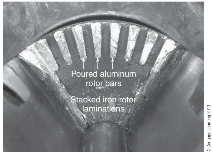
FIGURE 2-4 Poured rotor bars in iron laminations
