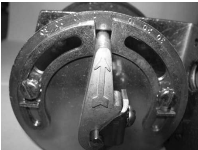
FIGURE 12-2 Float differential switch adjustment
