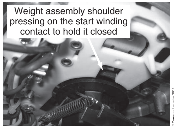
FIGURE 4-9 Weight assembly and start winding contact assembled
