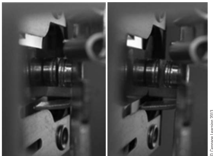
FIGURE 4-12 Start switch contacts open and closed
