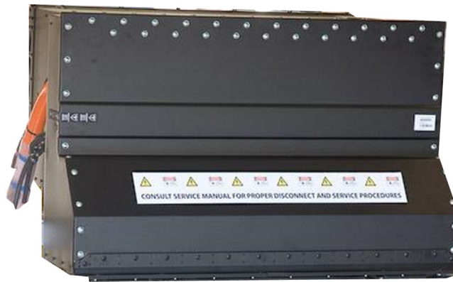
Figure 12 Tesla Roadster lithium-ion battery pack.
